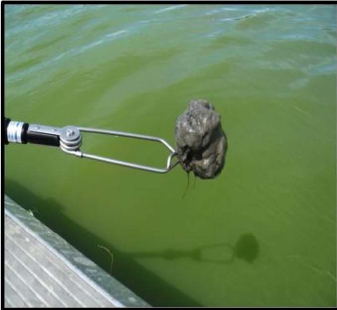
Figure 3. The grab sampler used to collect soft surface sediment from the lake bed.
