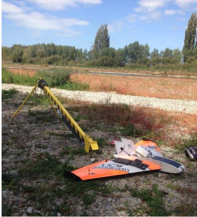
**Figure 1.** The fixed-wing UAV at the Opihi River shown with the catapult, which launches it.
