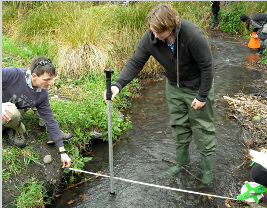
Water 402/602 students gauging water flow in Liffy Stream at Lincoln
